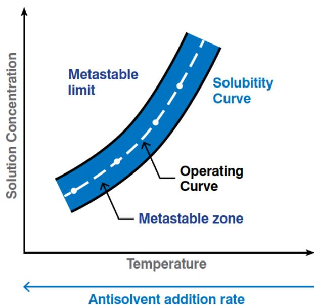
Fig 2: Schematic comparison of cooling vs. anti-solvent crystallisation.
