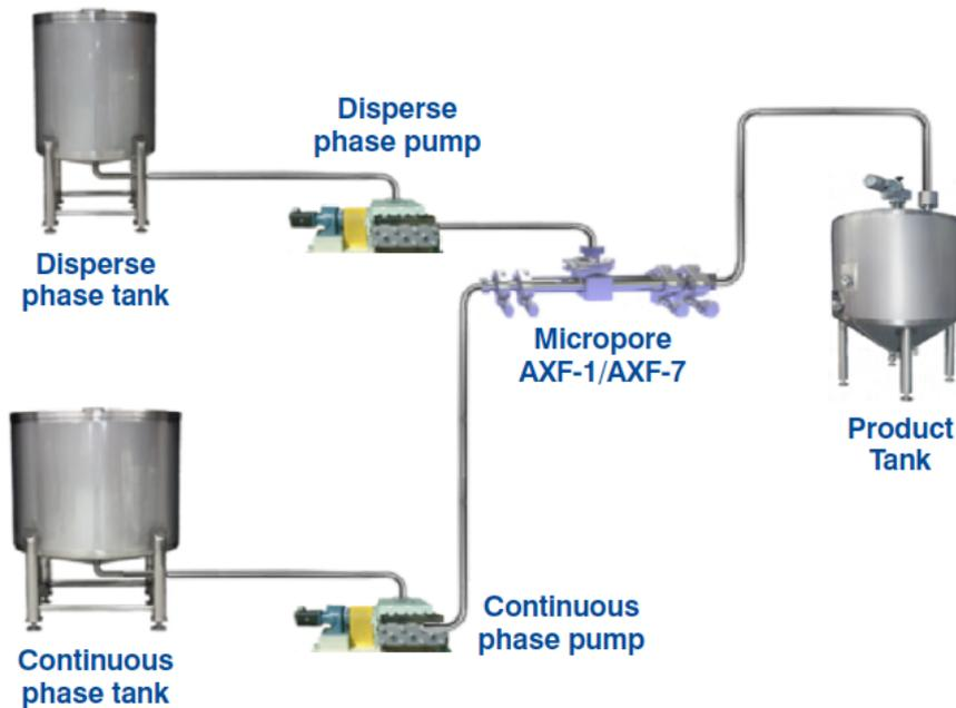
Fig 5: Schematic of Micropore crystallisation plant
